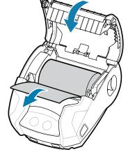
Close the media cover making sure to manually feed the end of the media roll outside the printer.
