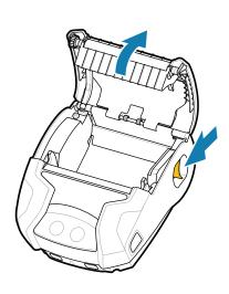
Slide the latch release forward to open the media cover.
