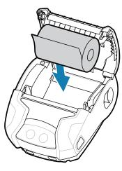
2. Insert the media roll in the media compartment in the orientation shown.
