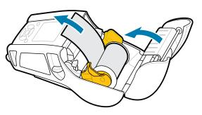
3. Close the media cover making sure to manually feed the end of the media roll outside the printer.
