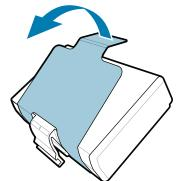
4. Peel back the tape insulator and remove it from the top of the battery pack. Discard upon removal.
