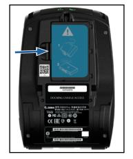
Rotate the pack away from the battery well. Lift the battery up and out of the printer.
