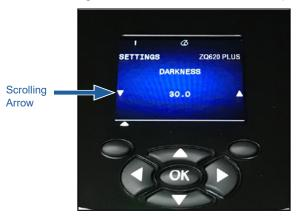
Some parameter settings, like Darkness, have a scroll option to view multiple setting choices. This option is identifiable by the presence of up and down scrolling arrows located on either side of the display (Figure 18). Press the **UP ARROW** and **DOWN ARROW** on the keypad to scroll through a menu's options. In some cases, further actions will appear on the right side of the status screen (see arrow in Figure 19). Press the **RIGHT SOFT KEY** to initiate said action.
