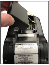
4. Rock the battery into the compartment as shown until it locks in place.
