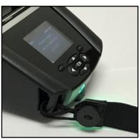
Loop the end of the strap back around the cut out and secure it over the button.
