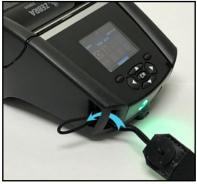
1. Insert the loop on the end of the strap through the cut out on the front of the printer as shown below.
