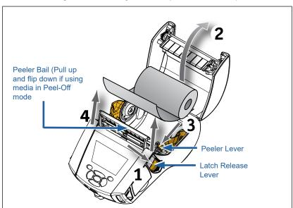
Figure 12 • Activating Peeler Bar (ZQ620 Plus Shown)
