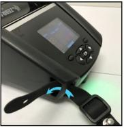
Insert the end of the shoulder strap behind the post on the front side of the printer and loop it around the post.
