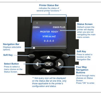
Figure 16 • LCD Control Panel
