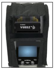
Slide the printer into the case such that the LCD display is visible through the plastic window.
