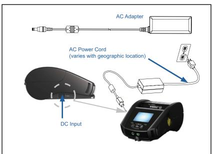
Figure 5 • AC Power Adapter Charging
