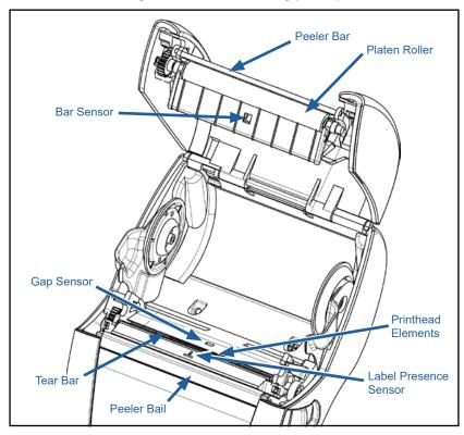
Figure 36 • ZQ6 Plus Cleaning (Linerless)
