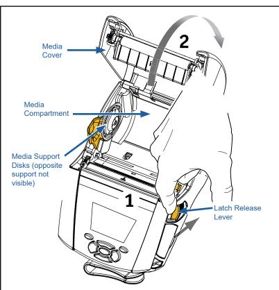
Figure 10 • Opening the Printer
