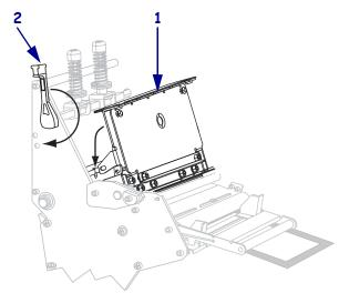
The backing winds on the rewind spindle or core.
