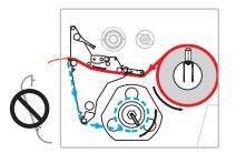
**8.** Remove the rewind plate (if installed) from the front of the printer. Store it on the two mounting screws on the inside of the printer base.
