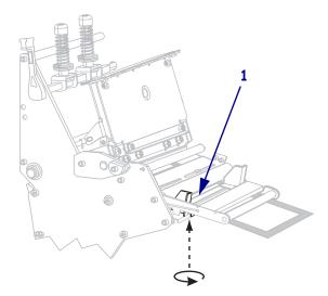
11. Push down the printhead assembly (1), and then rotate the printhead-open lever (2) until it locks into place.
