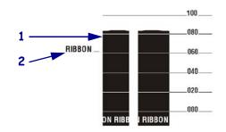
**Media Sensor Profile (Figure 20)** The media sensor readings are shown as bars and flat areas on the sensor profile (Figure 20). The bars (1) indicate gaps between labels (the web), and the low areas (2) indicate where labels are located. If you compare the sensor profile printout to a blank length of your media, the bars should be the same distance apart as the gaps on the media. If the distances are not the same, the printer may be having difficulty determining where the gaps are located.
