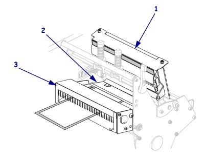
**9.** Align the media with the inner media guide (**1**). Slide in the outer media guide (**2**) until it just touches the edge of the media.
