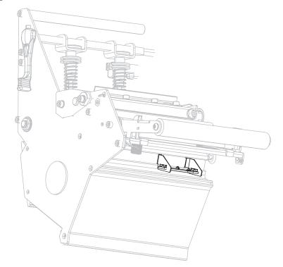
**2.** Slide the lower sensor until it is under the upper media sensor. Use the light that shines from the lower sensor to help align it with the upper sensor. Gently pull the wires as needed (wires should have a little slack).
