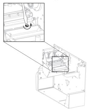
**3.** Using a thin, flat-blade screwdriver, loosen the upper media sensor adjustment screw.
