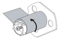
17. Align the media with the inner media guide (1). Slide in the outer media guide (2) until it just touches the edge of the media.
