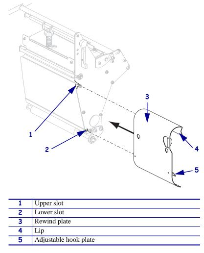
**10.** Insert the hook plate lip 1/2 in. (13 mm) into the lower slot in the side plate.
