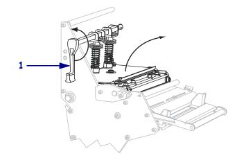
8. Thread the ribbon over the media dancer assembly (1) and under the ribbon guide roller (2).
