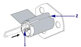
**b.** Rotate the spindle counterclockwise several turns to wind the media liner over the hook and remove any slack.
