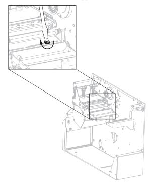
**5.** Tighten the adjustment screw to secure the upper media sensor in its new position.
