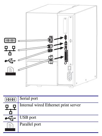
Table 4 on page 41 provides basic information about data communication interfaces that you can use to connect your printer to a computer. You may send label formats to the printer through any data communication interface that is available. Select an interface that is supported by both your printer and your computer or your Local Area Network (LAN).
