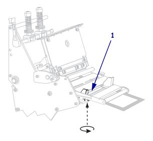
10. Push down the printhead assembly (1), and then rotate the printhead-open lever (2) until it
