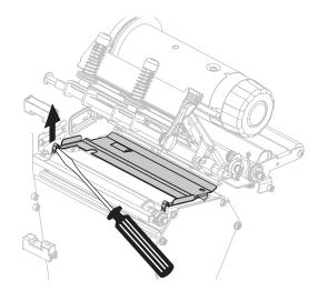
**4.** Insert the small-blade screwdriver or similar tool into the loop on the right side of the snap plate. Gently lift the right side of the snap plate.
