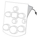
2. Carefully align the cover over the keypad. Press to make the cover adhere to the printer.
