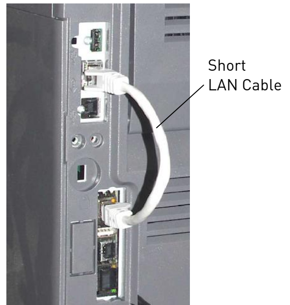
Fig. 5.1.b Detail: Establishing the LAN connection between the MPC and the basic engine
