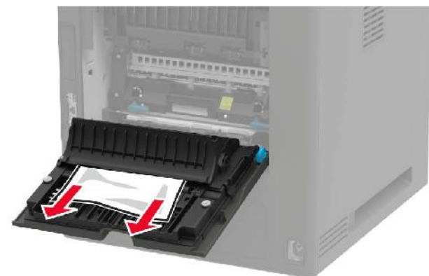
Fig. 11.4.5.d Removing jammed paper from the duplex area
