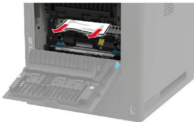
Fig. 11.4.5.b Removing jammed paper from the fuser area
