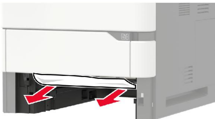
Fig. 11.4.2.b Pulling jammed paper
