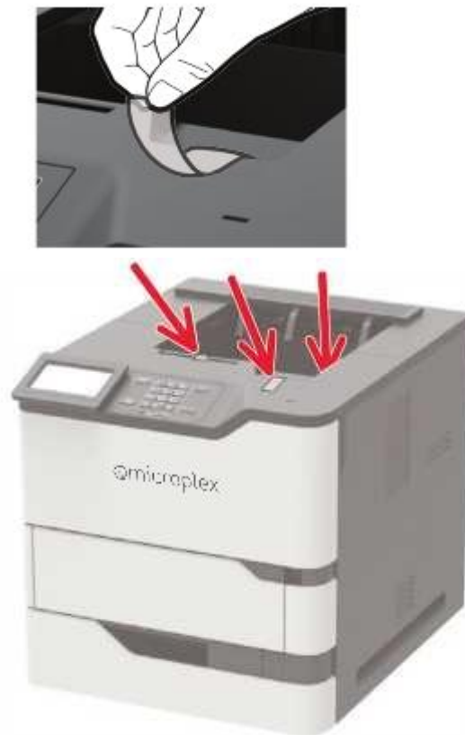
Fig. 2.2.c Removing the transport safety elements
