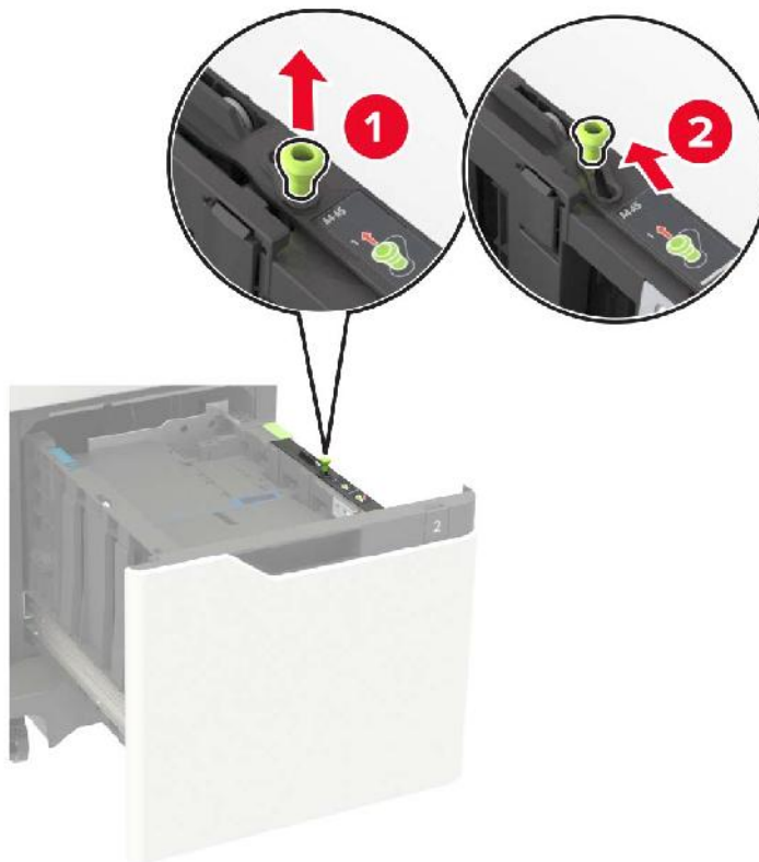
Fig. 4.1.2.a Pulling up and sliding the width guide to the correct position
