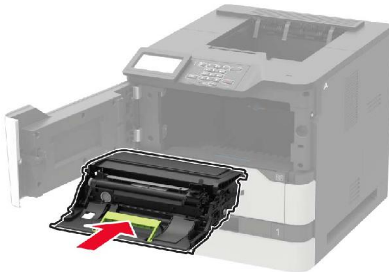
Fig. 4.3.g Sliding the new imaging unit into the printer
